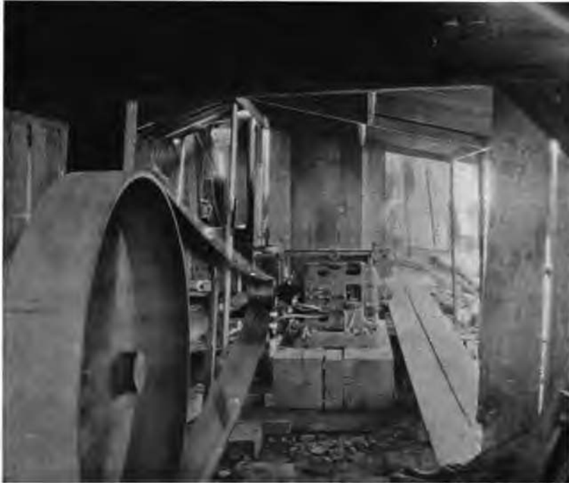
FIG. 53. Westinghouse motor belted for drilling.
