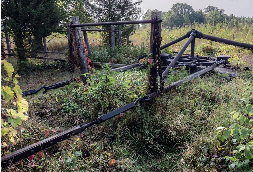
The unique system of jerker lines connecting the power to the pumps at Oil Springs, Canada (©AI Hayward).
