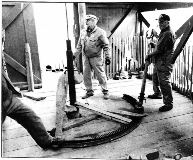
Men at Ontario Drilling Museum demonstrating the use of a well jack.
